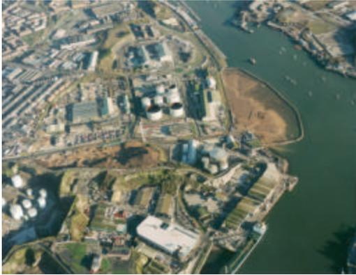
Cattedown Regeneration Scheme involves the excavation of 425,000 tonnes of limestone rock from a disused quarry and depositing it in Cattewater Estuary to form two six acre areas of development land.
